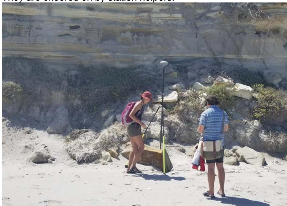
September 9 th , 2018. A portion of this trip was dedicated to collecting ground control points along the cliffs and beaches of Bechers with our RTK GPS unit. Students got hands on experience in the field with this advanced GPS technology.
