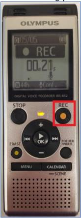
2. To pause the recording, press the record button again. Press again to continue the recording.
