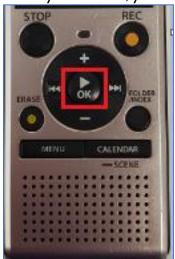
5. Press the + and – buttons (above and below OK) to change the volume of the recording playback. You may change the volume while the playback is in progress or while it is stopped
