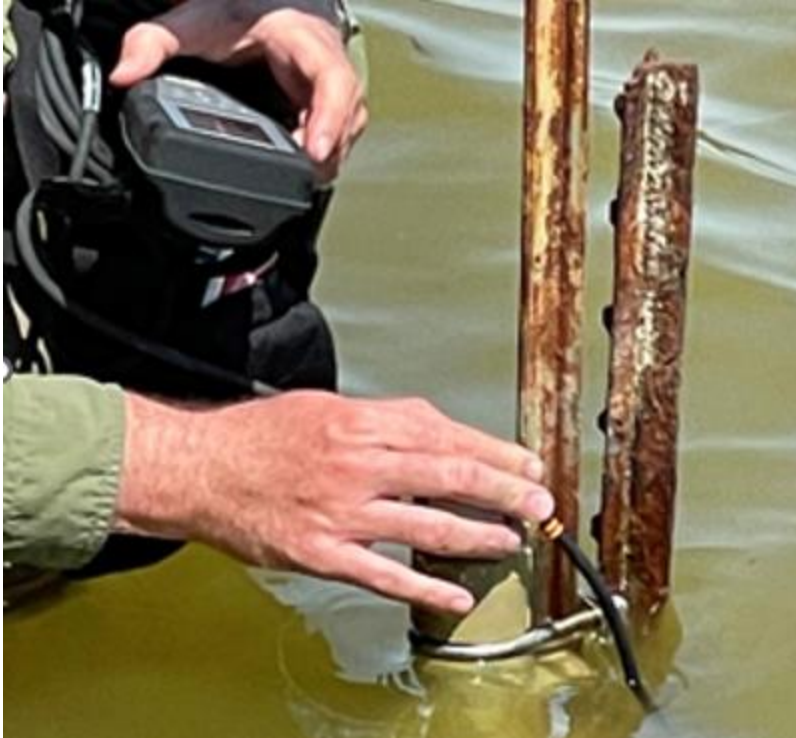
Figure 3. Housing and mounting apparatus for logger units, and SRIRS staff removing the top of the housing to read the logger. Also pictured is the YSI unit (left hand) used for calibration measurements.
