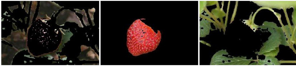
Figure 5. K-Means clustering: Divides the pixels into three clusters, grouping the most similarly colored pixels together and returns the separated clusters. Here is an example showing the three resulting segments for the sample strawberry image.
